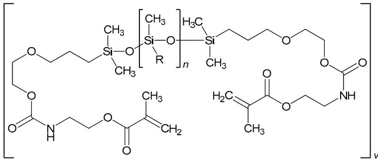
R = CH<sub>3</sub> (a) or CH<sub>2</sub>-CH<sub>2</sub>-CF<sub>3</sub> (b) or CH<sub>2</sub>-[CH<sub>2</sub>]<sub>2</sub>-[O-CH<sub>2</sub>-CH<sub>2</sub>]<sub>d</sub>-OCH<sub>3</sub> (c)
